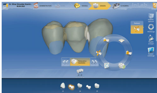
Fig 2 The inLab software enables the connectors to be manufactured as individual components and permits the restorations to be designed using various different tools.
